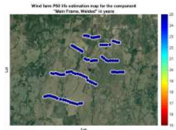
Figure 6.6: P50 Lifetime at main frame welded
