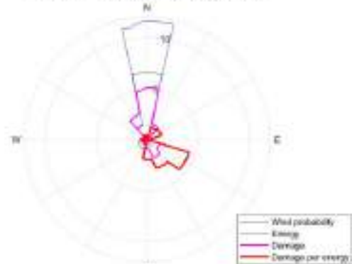
Rose map for the probabilities, energy and LTE for the component "Tower top" in percentage, WT81
