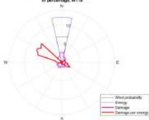
Rose map for the probabilities, energy and LTE in percentage, WT19
