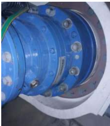
Figure 5.5: Oil leak and low oil level T18
