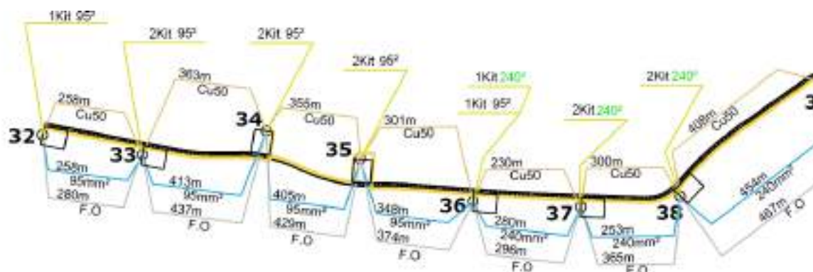
Figure 3.15: Underground Splices Detail
