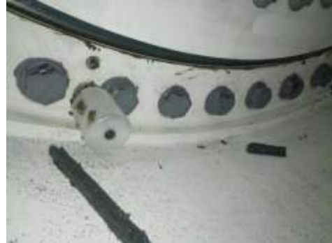
Figure 5.2: Lose torque mark T112
