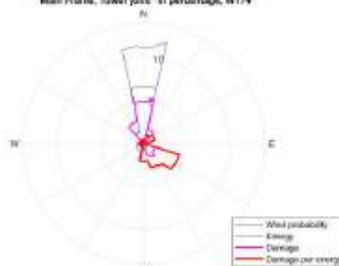
Rose map for the probabilities, energy and LTE for the component "Tower top" in percentage, WT74
