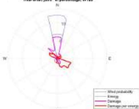
Rose map for the probabilities, energy and LTE for the component "Hub-Shaft joint" in percentage, WT23
