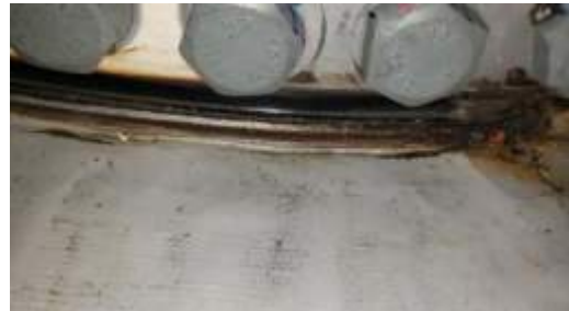
Figure 5.4: Grease bearing leakage T59
