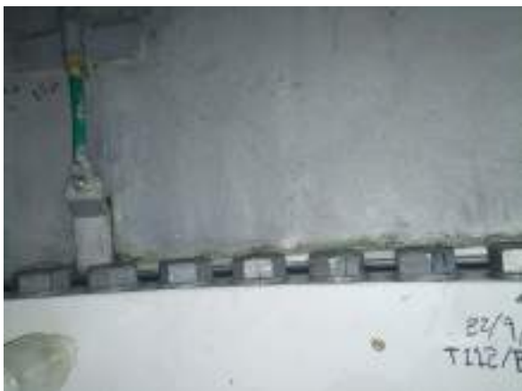
Figure 5.9: Lose torque mark in blade bolts
