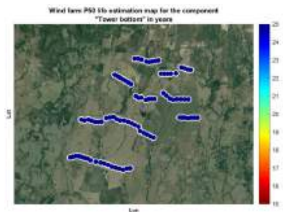
Figure 6.9: P50 Lifetime at tower bottom
