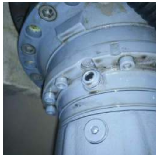
Figure 5.6: Oil leak and low oil level T63
