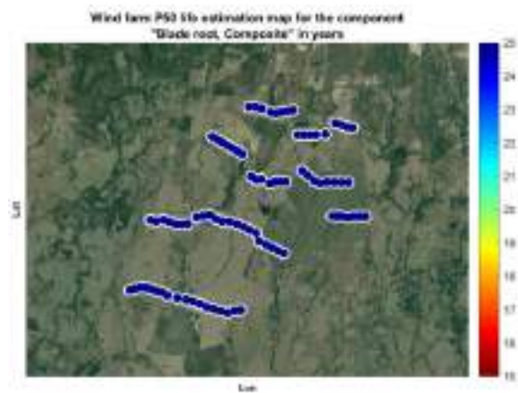
Figure 6.1: P50 Lifetime at Blade root composite
