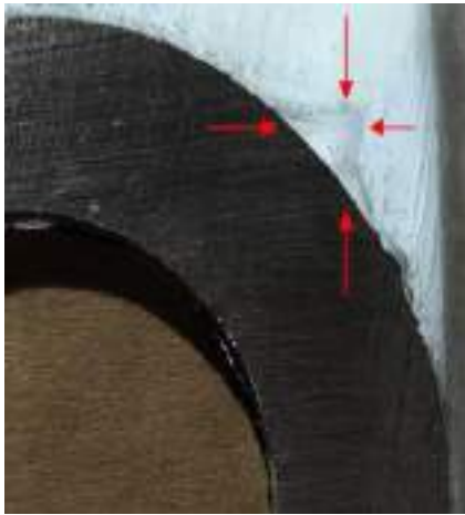
Figure 5.11: Void in the blade insert
