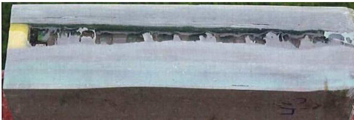
Figure 4.4: Examination of root bushing from blades at UEP II
