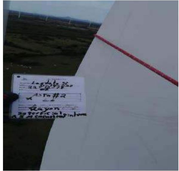
Figure 6.8: T7 Superficial Scratch
